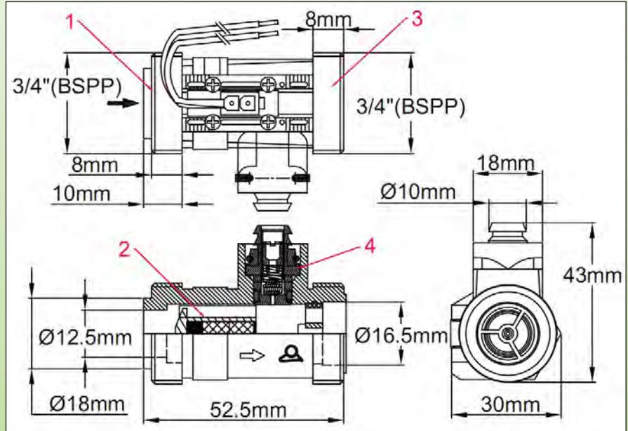
**Main applications:** Product developed for electrical or gas instantaneous water heaters. 3/4" BSPP male water inlet and outlet. Mandatory vertical mounting, with water inlet from the bottom. **Built-in over-pressure valve**
