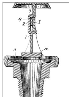
1890: Grinnell sprinkler head using parts welded together with a fusible alloy and a leveraging effort mechanism
